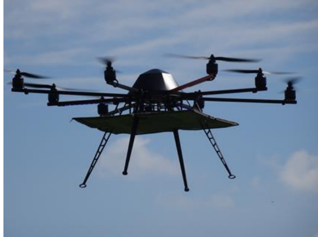
Figure 45: Picture of the Okto-XL ARF-Mikrokopter flying over Dourbes. This UAV will be equipped with a transmitter developed at BIRA-IASB so as to act as a known radio source in the far field of the antennas.
