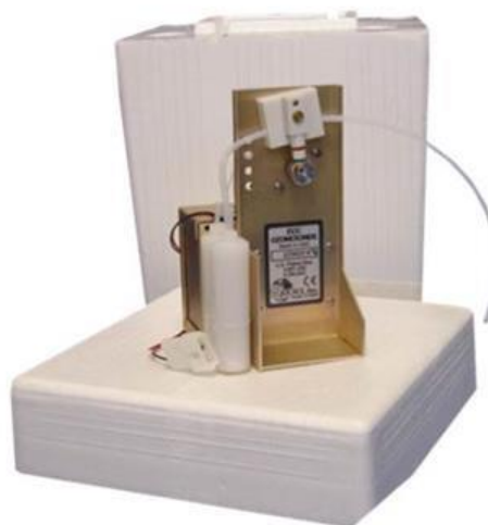
Figure 36: Photograph of the Electrochemical Concentration Cell (ECC) ozonesonde used at the Royal Meteorological Institute
