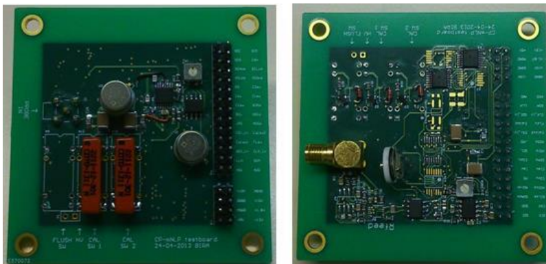
Figure 46: Pictures of the capacitive feedback electrometer prototype board (1 channel)
